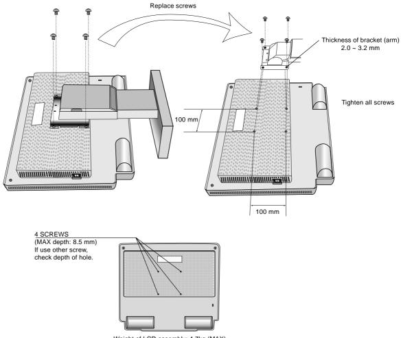
Weight of LCD assembly: 4.7kg (MAX)
